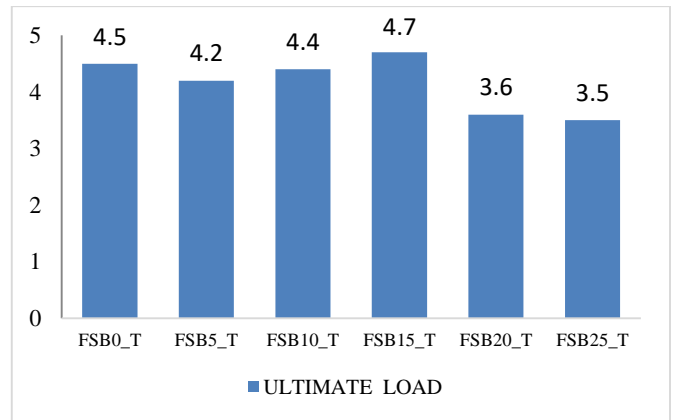
Figure 6. Ultimate load of three layered slabs
